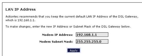
The values in the “Modem IP Address” and “Modem Subnet Mask” text boxes are the IP and subnet mask address of the Gateway as seen on the network. These values can be modified for your LAN network, but we recommend keeping the default factory settings (IP address 192.168.1.1; subnet mask address 255.255.255.0).
