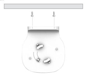
5. There are two mounting slots located on the bottom of the Fios Router. It allows you to securely attach your router to the wall. Align the slots with the wall mount bracket.
