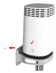
8. To secure the bracket, place one screw into the small hole of the bracket and tighten the screw into your wall.
